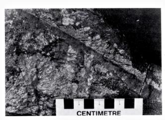
Fig. 23. Dendritic feldspar showing curved growth morphology. Convex, lattice planes can be recognized from the weakly discolored, transverse pattern on the feldspar stem. The crystal measures 18 cm. Secondary nucleation of pyroxene and nepheline on the upper surface tends to readjust growth towards the maximum heat flow.
